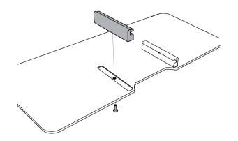
Insert the attached work surface track into the plastic guide on the column arm.
