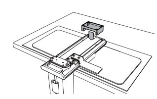
The Tycho allows you to align the keyboard try to the left or right for better ergonomic
