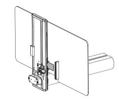
Insert the unattached work surface track into the opposite plastic guide on the column arm and attach using the screw you removed in step one.
