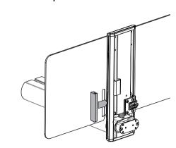
Rest the unit upside down over the edge of a desktop or work surface on top of cardboard divider (marked with "B" in packaging).
