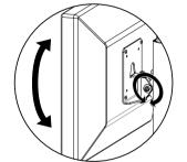
Note: To adjust the forward/ backward tension of the VESA mount, loosen or tighten the tension bolt with the included hex key and wrench. Do not do this until you have mounted the monitor(s) on the base unit.
