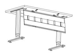
2. Install the hanging brackets with the hook sides facing inward using the ST4.8x19 screws into the hole positions marked in step 1.
